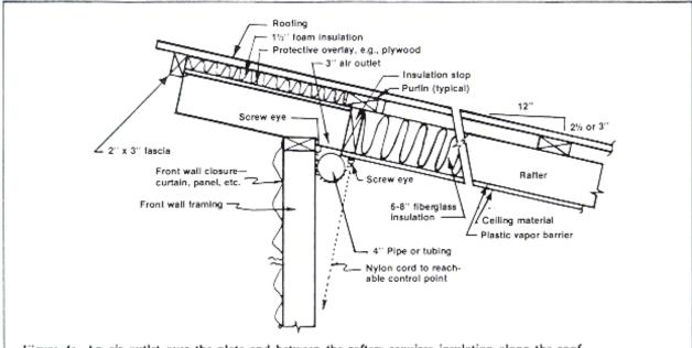
Figure 4a. An air outlet over the plate and between the rafters requires insulation along the roof and a narrow fascia.
