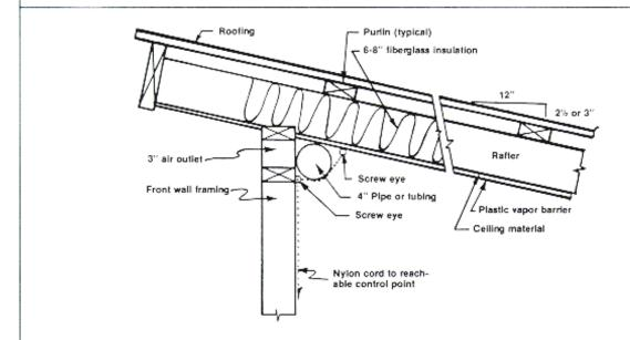
Figure 4b. An air outlet using a double plate to form a thru-the-wall opening.
