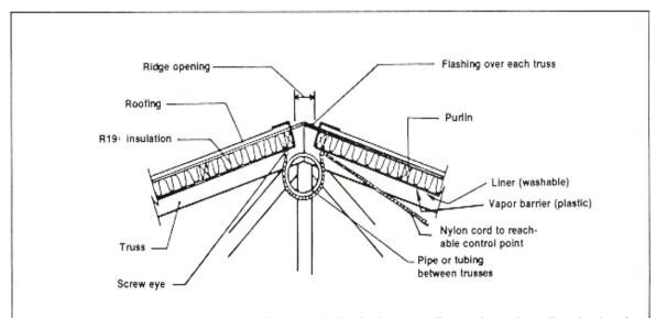
Figure 6. Ridge openings for a gable roof building. A plastic pipe in a rope sling can be used to adjust the size of a ridge opening. Install flashings along ridge and over each truss to prevent precipitation and condensation from wetting insulation and structural members.
