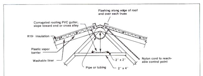
Figure 7. An interior trough or rain gutter can be added to an open ridge to intercept precipitation and prevent wet floors.
