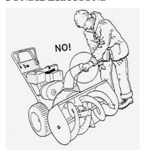
Most snow thrower injuries happen when consumers try to clear snow from the discharge chute or debris from the auger/collectors. **Keep hands and feet away from all rotating and moving parts.** Stop engine and wait for everything to stop and then use a long stick or shovel handle to clear blockages.
