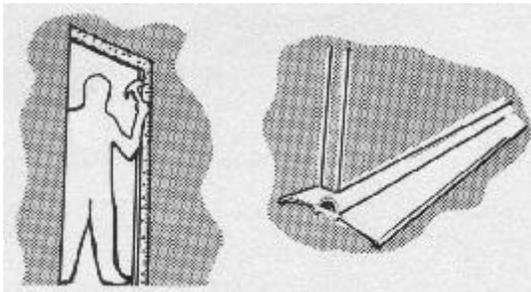
Window weatherstripping is attached to the window frame. On gliding or double hung windows weatherstripping needs to also be installed where the movable and fixed portions meet.
