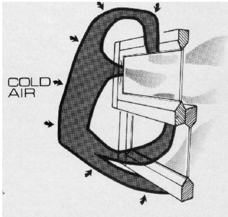
Caulk is used around outside window and door frames, and to fill outside wall and foundation cracks.
