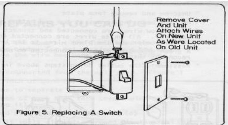
Wall Switch - When the light is out, first replace the bulb with one you know will light. With the new bulb in the socket turn on the switch. If light doesn't go on, check the fuse box in the basement. If fuses are all good the problem is probably the switch.
