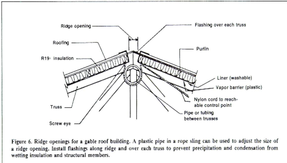
Figure 6. Ridge openings for a gable roof building. A plastic pipe in a rope sling can be used to adjust the size of a ridge opening. Install flashings along ridge and over each truss to prevent precipitation and condensation from wetting insulation and structural members.
