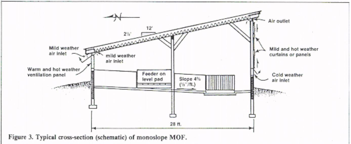
Figure 3. Typical cross-section (schematic) of monoslope MOF.
