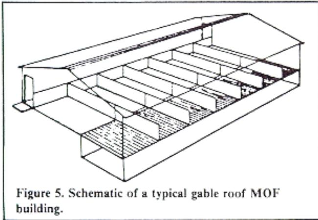
Figure 5. Schematic of a typical gable roof MOF building.
