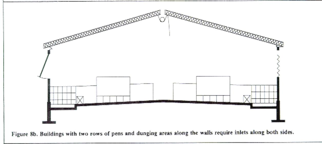
Figure 8. The location of inlets in a gable roof MOF is dependent upon the number of rows of pens and location of the dunging area(s).
