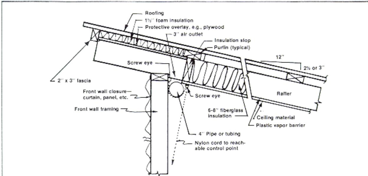
Figure 4a. An air outlet over the plate and between the rafters requires insulation along the roof and a narrow fascia.
