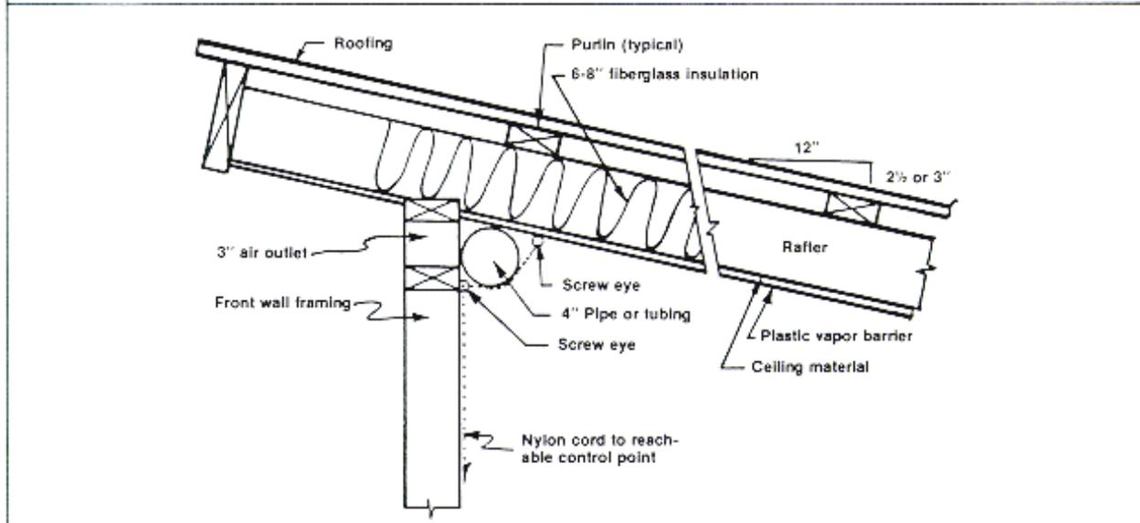
Figure 4b. An air outlet using a double plate to form a thru-the-wall opening.
