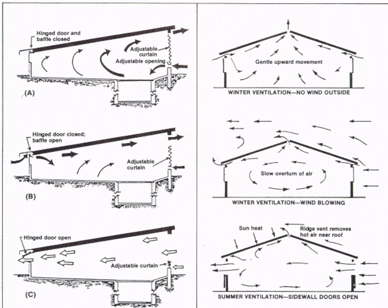
Figure 1a. Expected airflow patterns in a monoslope-roof building for (A) extremely cold weather, (B) mild weather and (C) hot weather.
