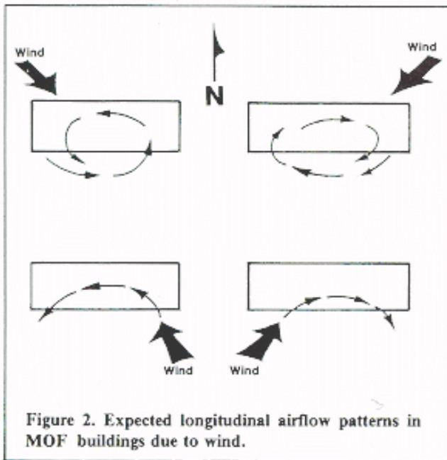
Figure 2. Expected longitudinal airflow patterns in MOF buildings due to wind.
